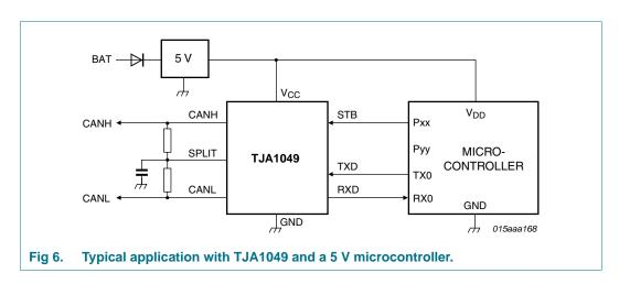
High-speed CAN transceiver with Standby mode
